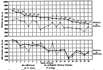
Fig. 19.—Effect of "boiling process" of preservative treatment on the strength and stiffness of Douglas-fir stringers treated green and tested without seasoning.
